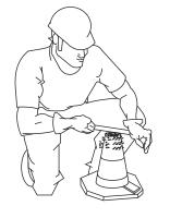
Figure 35-D. Slump Test (Removing Excess Concrete)
